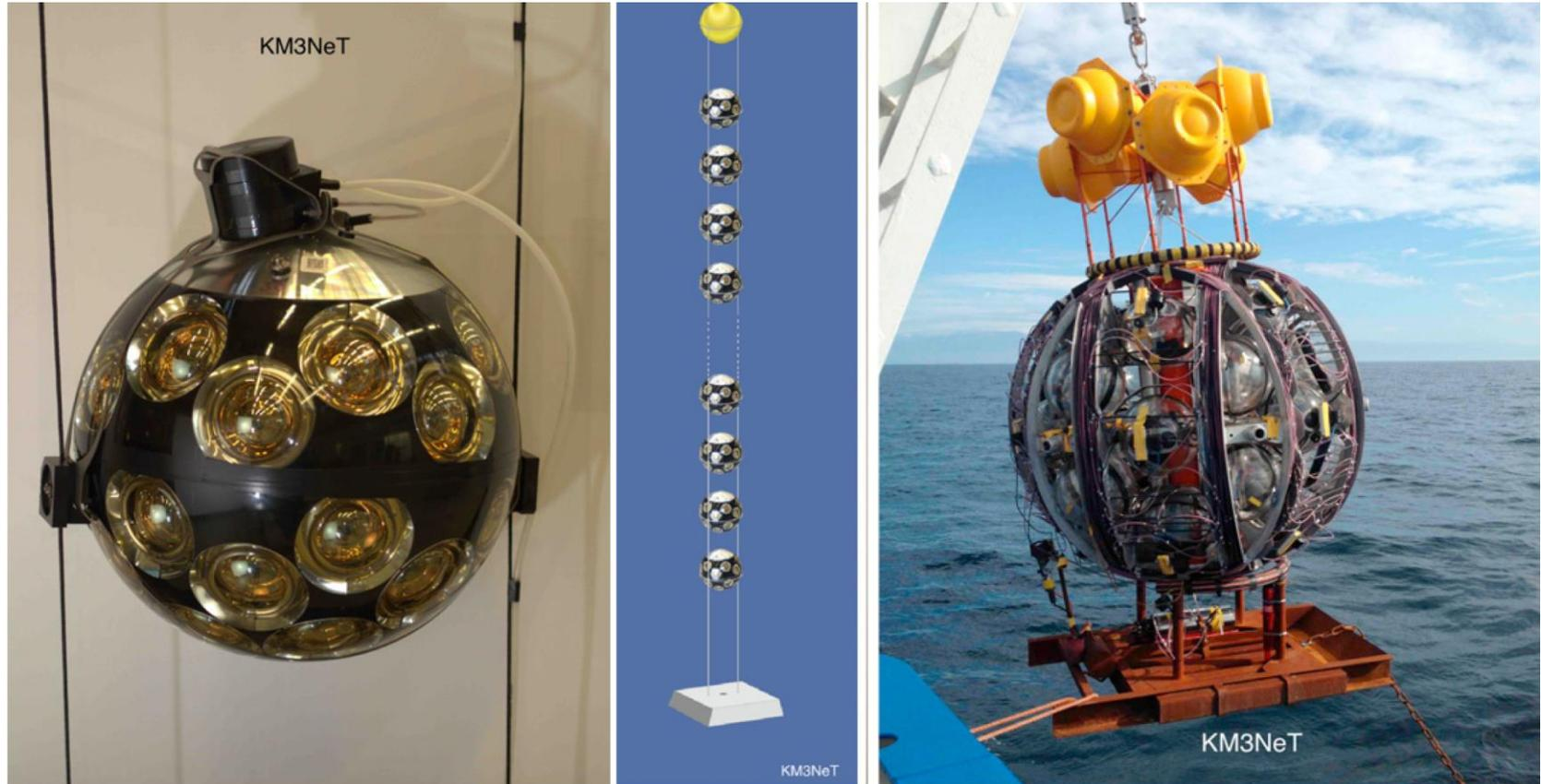
*The KM3NeT Digital Optical Modules (DOMs) and Detector Units (DUs).*
